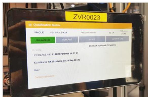
*Logging employee onto the production line and then displaying the status of the required qualifications*
